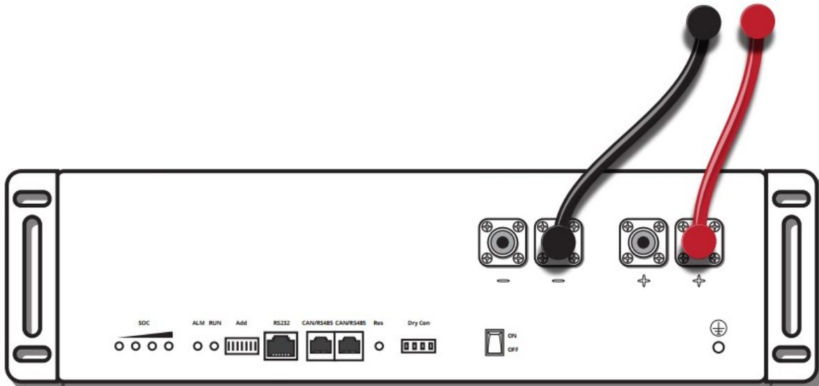
Figure 5 - Single Unit Connection
